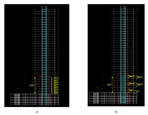
Figure 3. Models for sensitivity study of RC shear wall discretization: a) Model 1, b) Model 2.
