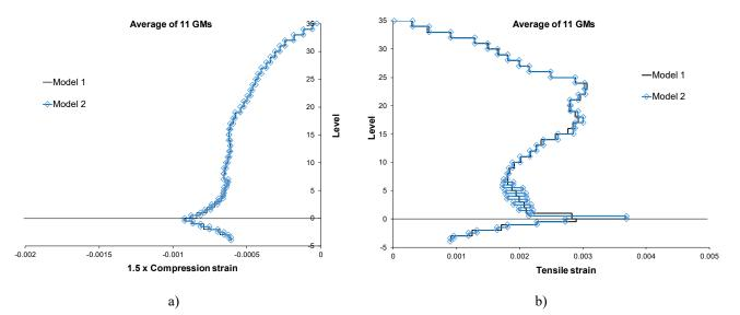
Figure 4. Average demand profiles for corner strain gage: a) Compression strains, b) Tensile strains.
