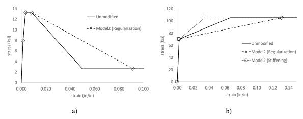
Figure 6. Modified stress strain curves using Regularization: a) Confined concrete stress strain, b) Reinforcing Steel
