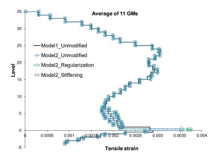
Figure 7. Average tensile strain demand profiles of modified and unmodified wall models.
