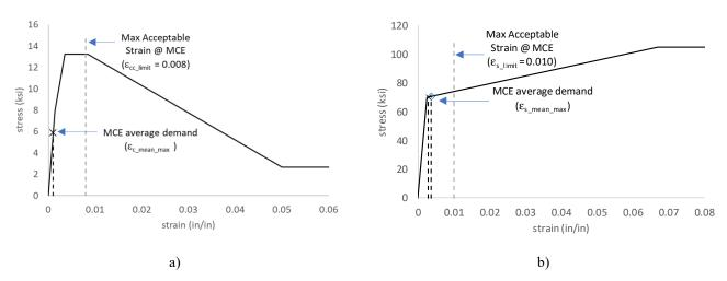
Figure 5. Maximum strain demands vs stress strain backbone curves: a) Confined concrete, b) Reinforcing steel.
