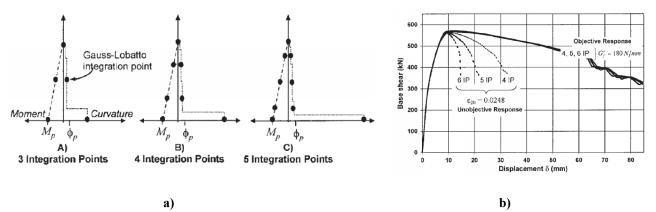
Figure 1. Localization of Inelastic Models with Varying Number of Integration Points (Coleman and Spacone, 2001), a) curvature profiles b) pushover predictions using unregularized and regularized material models
