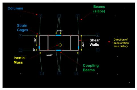
Figure 2. Structural plan view of reinforced concrete shear wall coupled wall system.
